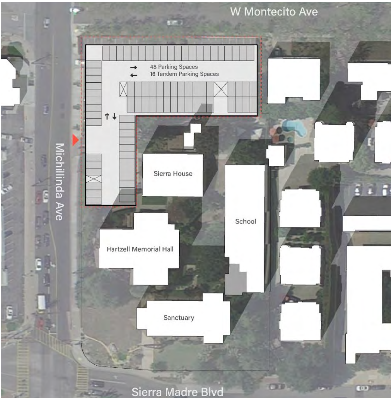
Figure 1 UMC Campus & First Floor Parking Plan
