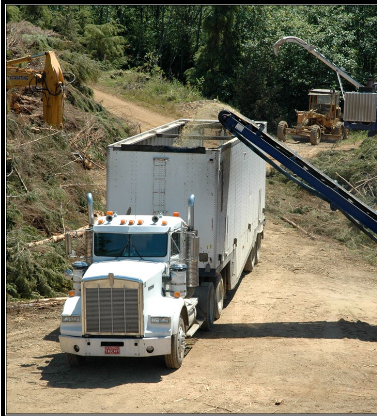
Figure 4.7 – Chip Van Being Loaded to Transport Biomass Fuel
